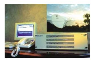
A Demand Assigned Multiple Access (DAMA) system is typically a single hop satellite transmission network which allows direct connection between any two nodes in the network among many users sharing a limited "pool" of satellite transponder space
