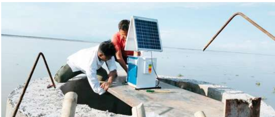
▼ Fig. 1.4: Jaltarangini – a flood forecasting and early warning system developed by NIC Assam – being tested in the Brahmaputra River in Dibrugarh.
