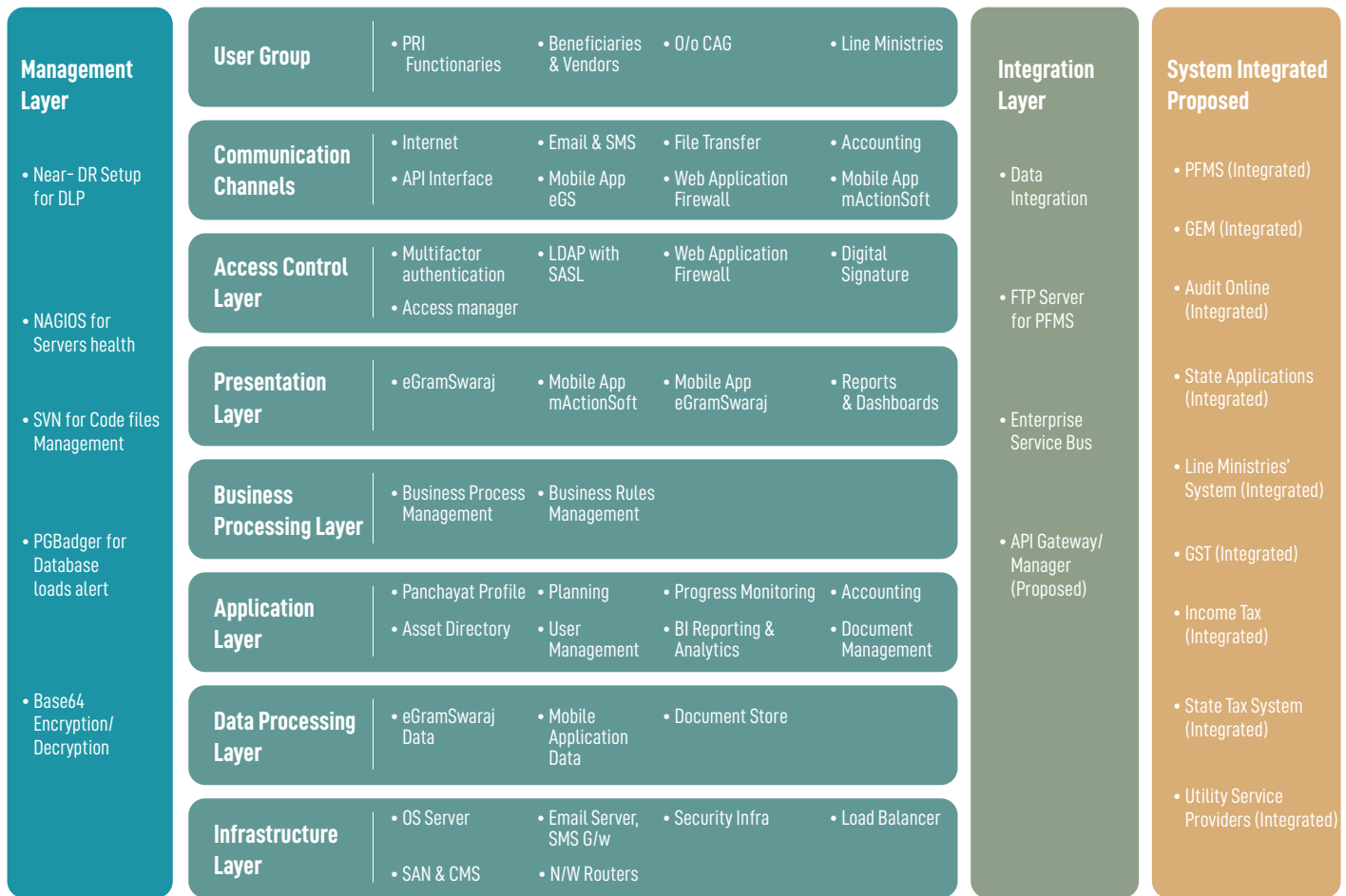
▲ Fig 9.5 Functional architecture and various components of eGramSwaraj application
