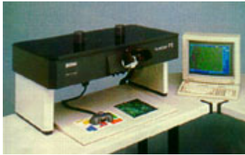
A P3 Analytical Stereo Plotter used by the NIC Utility Mapping Group
